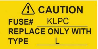
Fig 2. To maintain the proper SCCR rating, any fuses that must be replaced have to be the same type and rating as the original fuse. In this case, a simple label that identifies the replacement fuse is critical to maintain the system.
