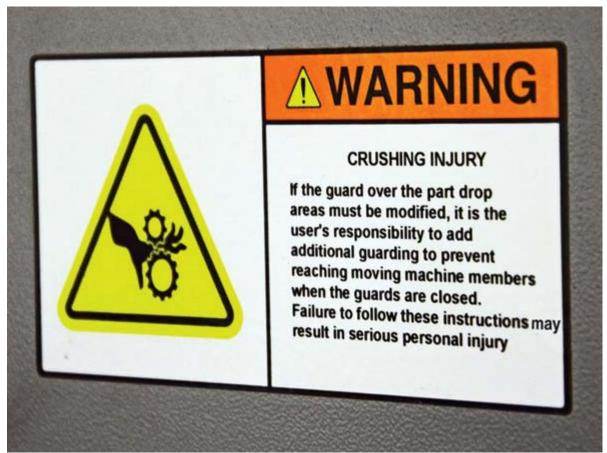
Photo 6. Pictograms can be used to identify hazards visually within the warning label.
