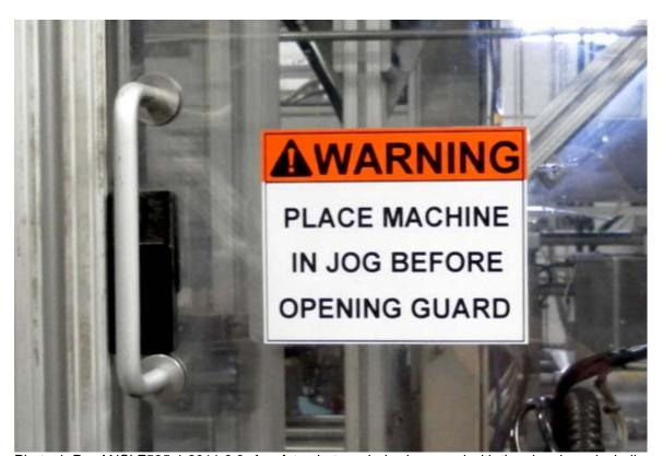
Photo 4. Per ANSI Z535.4-2011 6.3: A safety alert symbol, when used with the signal word, shall precede the signal word.
