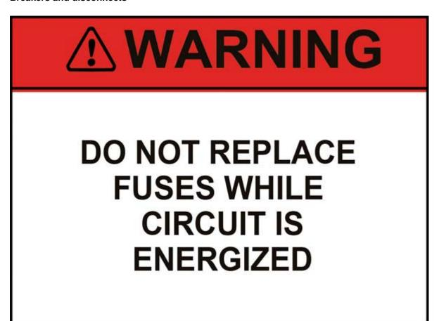
Fig. 3. If one has a medium-voltage substation in a facility, then this label would be placed on anything 600V or higher. Anything under 600V has the fuses contained in some type of disconnecting means that will automatically turn off power if the user attempts to access the fuses.
